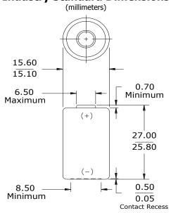
This battery contains a Positive Temperature Coefficient (PTC) safety device to limit current during short circuit conditions.
